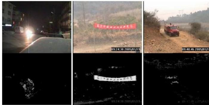
Fig. 11. Segmentation results of fire colored objects
