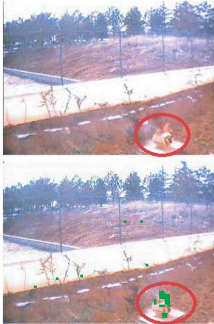
Figure 4. Flame detection in video. Initial video snapshot (top) and flames (green blocks) detected in primitive phase..
