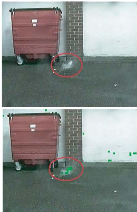
Figure 5. Smoke detection in video. Initial video snapshot (top) and smoke (green blocks) detected in primitive phase.
