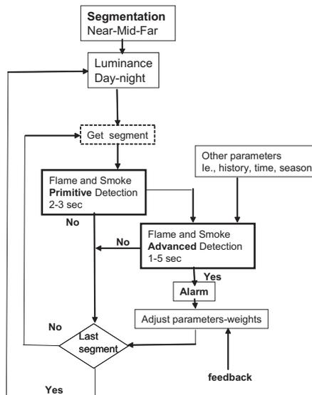
Figure 1. Fire detection subsystem flowchart
