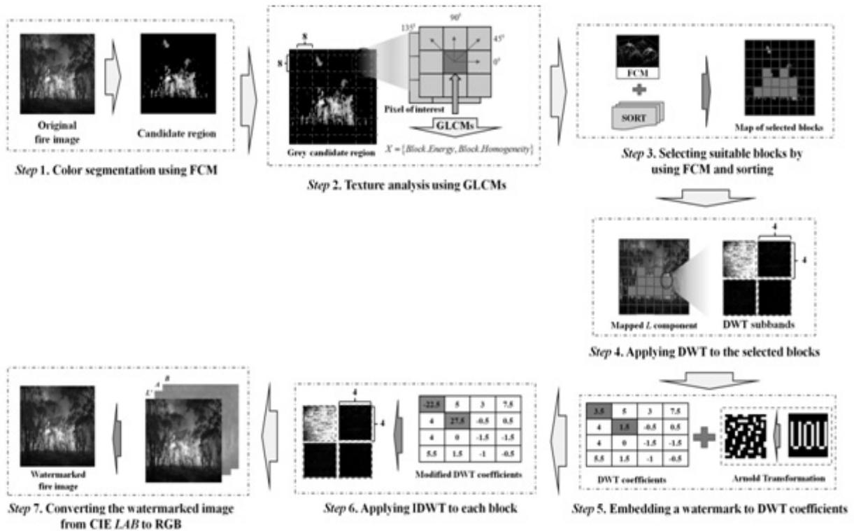
Fig. 3. Watermark embedding process of the proposed approach
