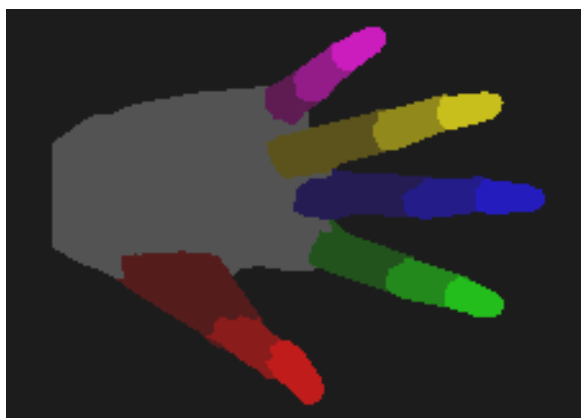
Figure 1: The hand as an articulated object. The palm and each finger are shown in a different color. The three different links of each finger are shown using different intensities of the same color.
